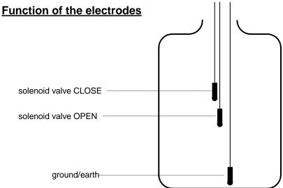
In normal operation, the water level varies between the "solenoid valve CLOSE" and "solenoid valve OPEN".
